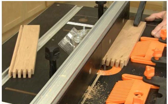
Step 27: Plowing a full-length groove in a drawer side at the router table
