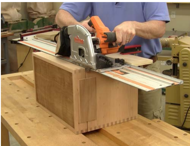
Step 19: Making the final long kerf cut to separate the lid from the chest carcass with a track saw
