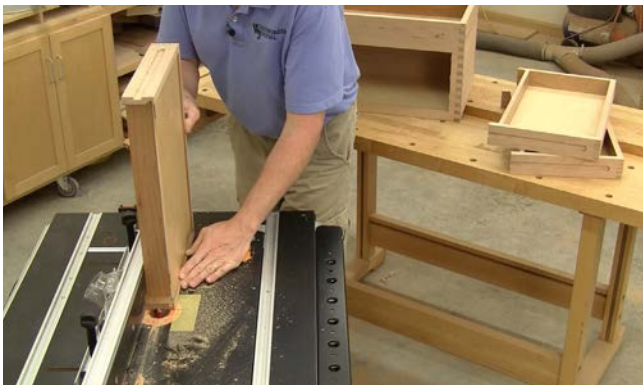
Step 35: Cutting stopped grooves on the sides of the drawers to fit over the chest's plastic drawer slides
