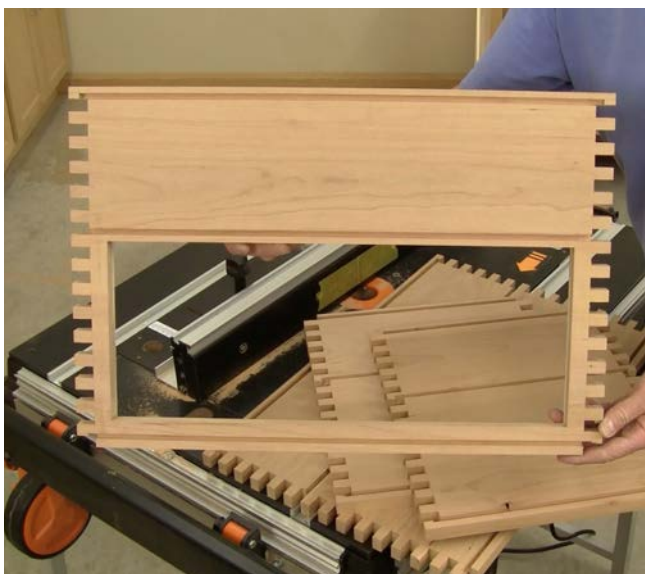
Step 9: Showing the three groove cuts made in the front panel
