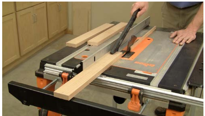
Step 23: Ripping the remaining blank from the project's front panel into three drawer faces
