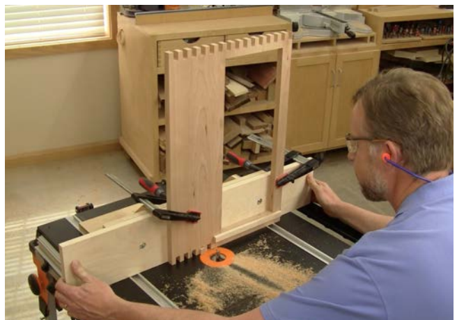
Step 7: Cutting box joint pins and slots on the front panel of the chest
