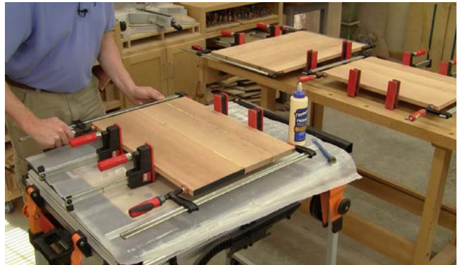
Step 1: Spreading glue and clamping up a panel on the Clamping Module
