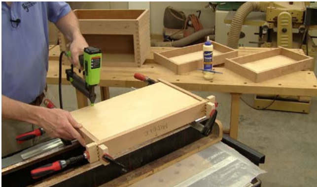
Step 33: Installing drawer bottoms on the drawers with brad nails
