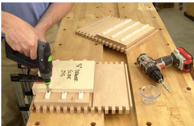
Step 14: Screwing the slides in place on the side panel filler pieces
