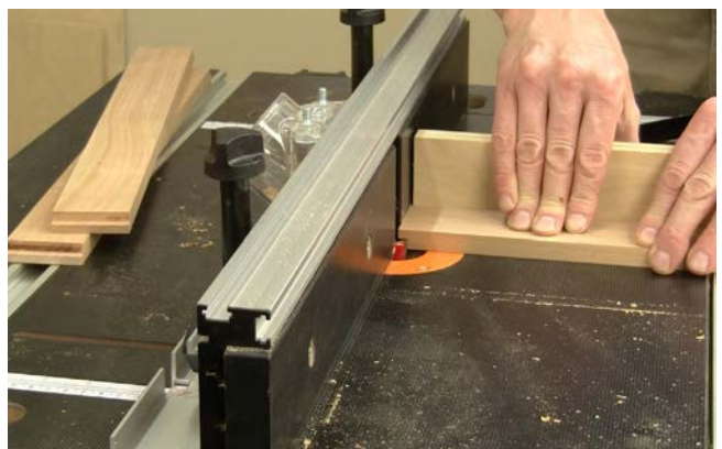
Step 29: Close-up of making two rabbeting passes on one of the drawer backs
